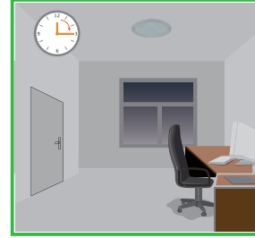
Light switches off automatically after the dimming time elapsed.
